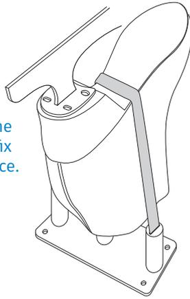
**2** Position blade on boot. The toe plate should be set approximately 1,5 mm back from the front of the boot sole.
