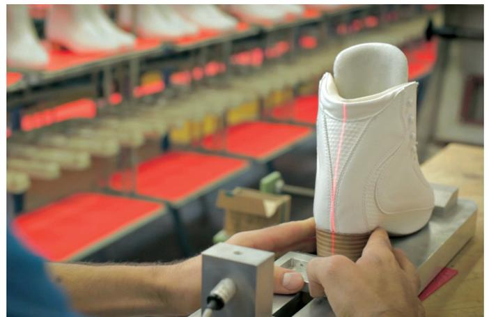
Laser control, to check if the sole and the upper are aligned
