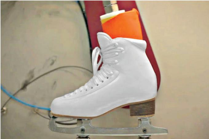
Flex testing machine, for long life test and stiffness measurements
